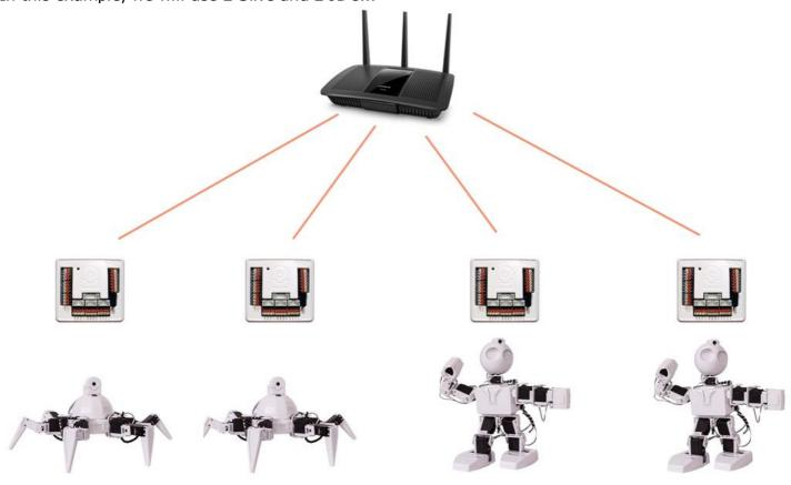
**Web Config** What you will need is a configured WiFi router. Keep note of the WiFi SSID Network name and the password. These two pieces of information will be entered into each EZ-B's web configuration tool.
