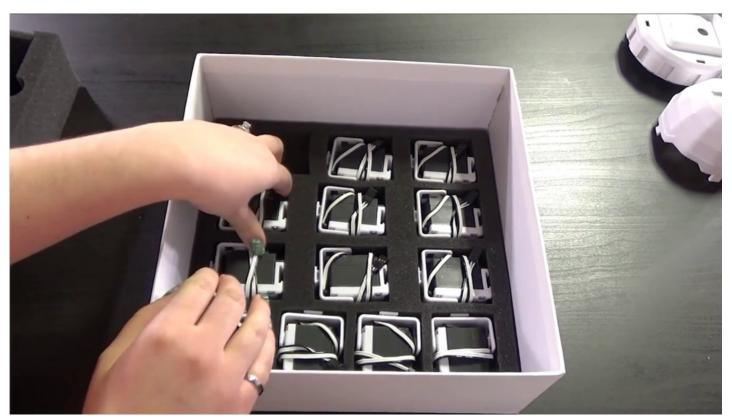
**Lever Servos** are a type of motor that can be controlled for specific positions. They act as joints for robot movement.
