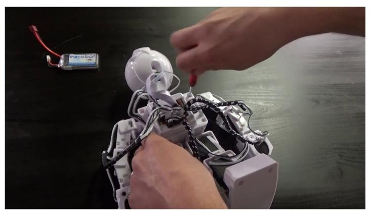
Screws do not need to be fully removed from the assembly.
