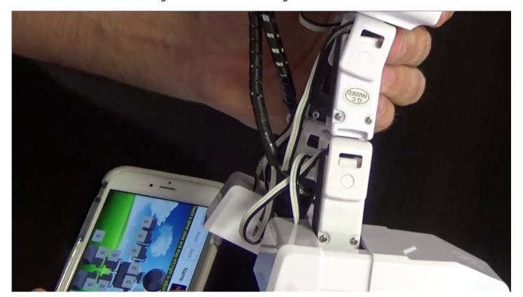
Adjust the software servo values to line up each servo. Start with the servos closest to the body and move outwards.
