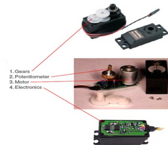
Figure 5. The circuit board and DC motor are in a high-power servo. Did you notice how few parts are on the circuit board? Servos have evolved to a very efficient design over many years.
