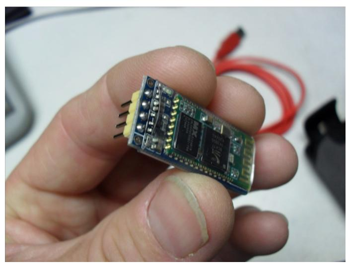
2. I used the <u>male jumpers</u> that I got from the EZ Robot Store to hook up the FTDI header to the EZ-B header. <del>VCC to VCC <- EDIT: Found out this connection is not needed.</del> GND to GND Tx to Tx Rx to Rx (Yes that's right Tx to Tx and Rx to Rx. I thought it should be Tx to Rx and Rx to Tx but that did not work.)
