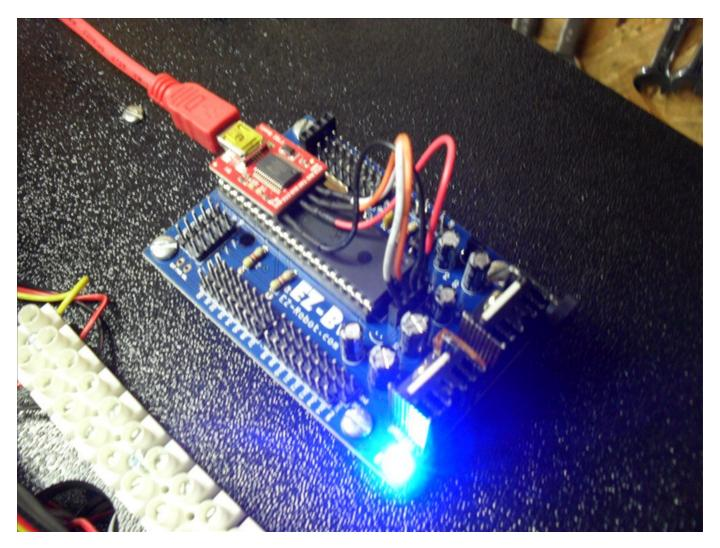
Notice anything interesting in the picture above?..... When I unhooked the battery pack from the EZ-B the EZ-B remained on. It was being powered from the Mini ITX. **Connection was not lost**. The blue LED remained on. However, I found that the servo would not work anymore until I hooked the EZ-B battery pack back up.
