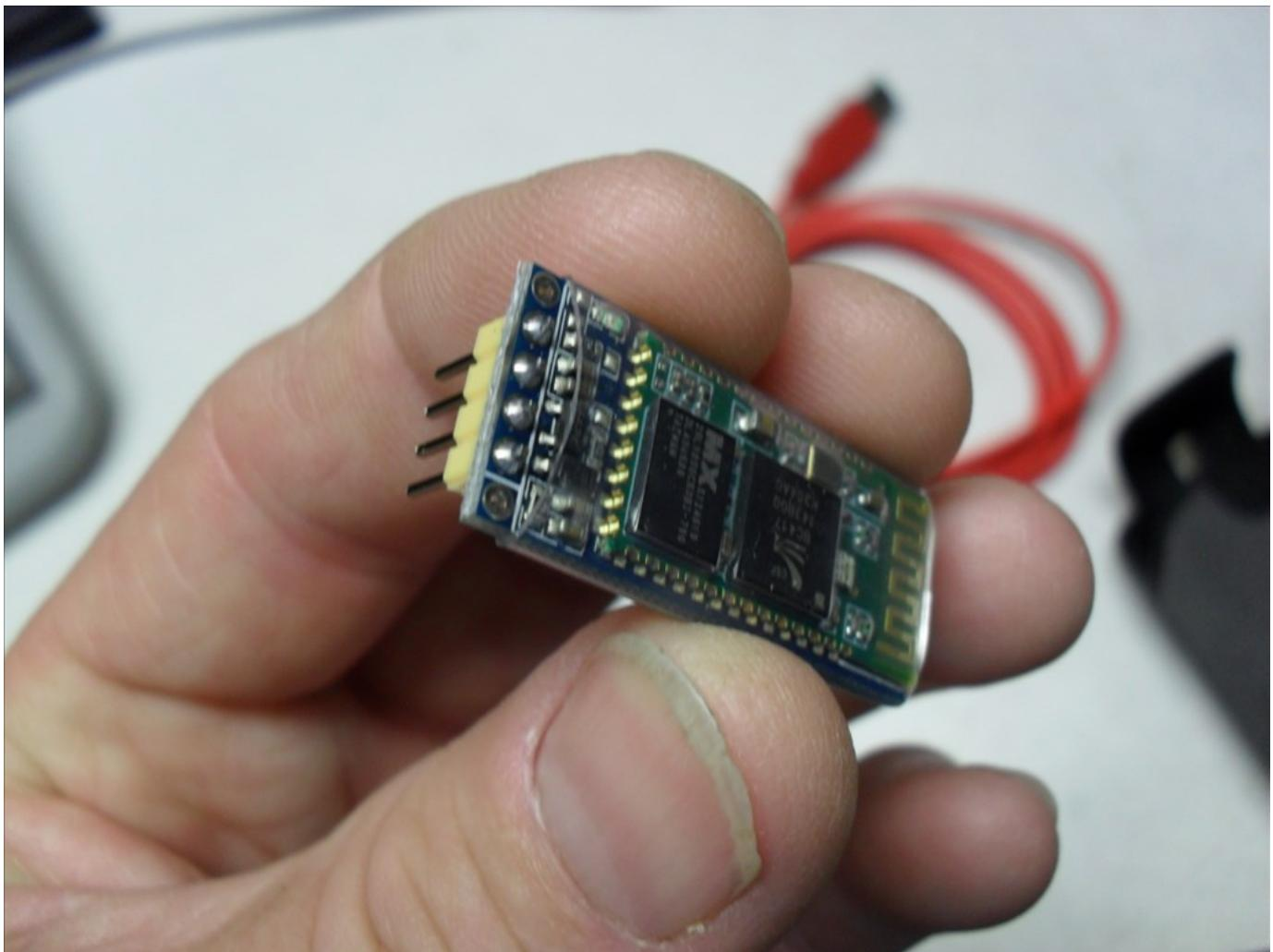
2. I used the [male jumpers](#) that I got from the EZ Robot Store to hook up the FTDI header to the EZ-B header. VCC to VCC <- **EDIT: Found out this connection is not needed.** GND to GND Tx to Tx Rx to Rx (Yes that's right Tx to Tx and Rx to Rx. I thought it should be Tx to Rx and Rx to Tx but that did not work.)
