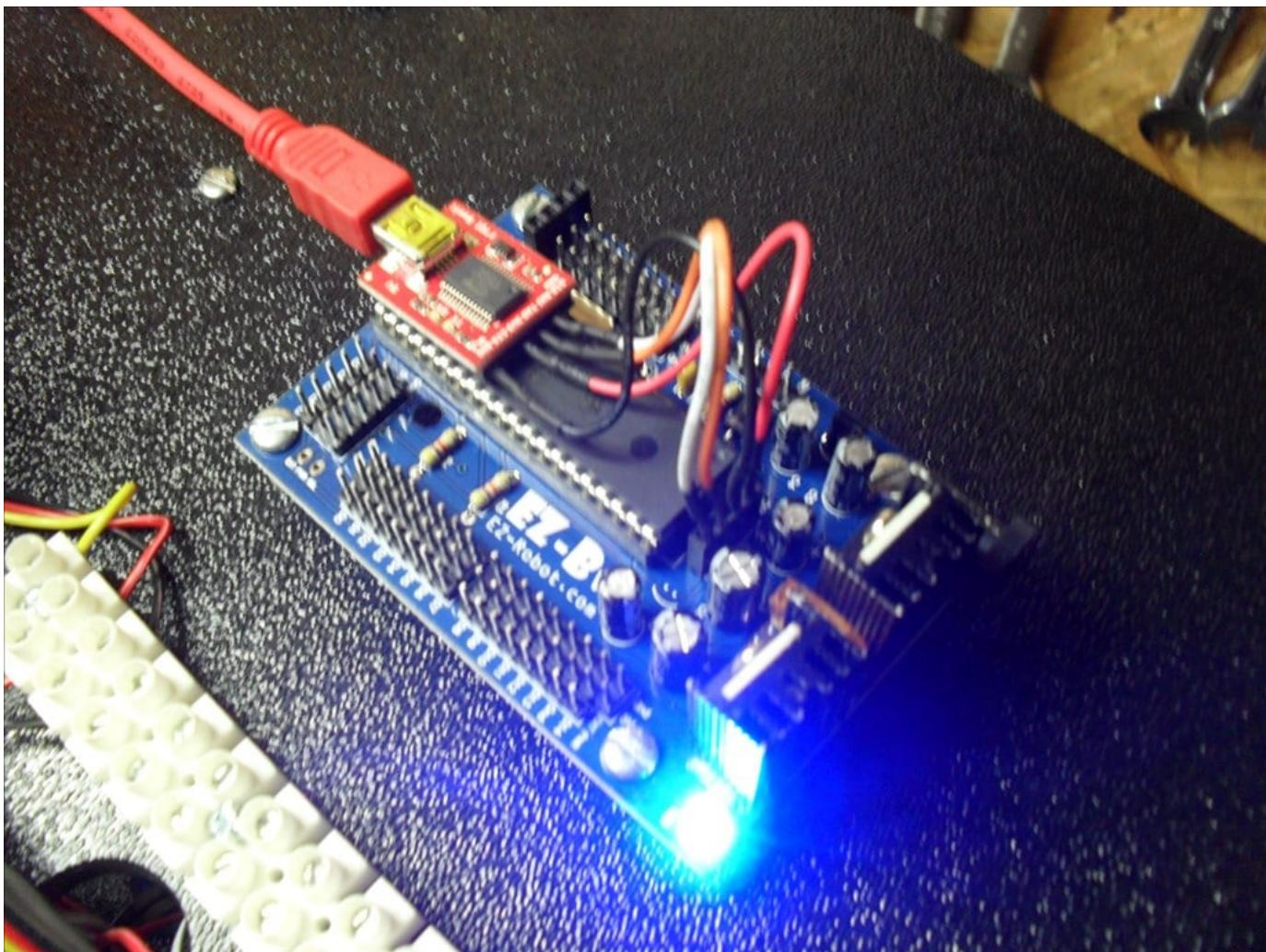
Notice anything interesting in the picture above?..... When I unhooked the battery pack from the EZ-B the EZ-B remained on. It was being powered from the Mini ITX. **Connection was not lost.** The blue LED remained on. However, I found that the servo would not work anymore until I hooked the EZ-B battery pack back up.
