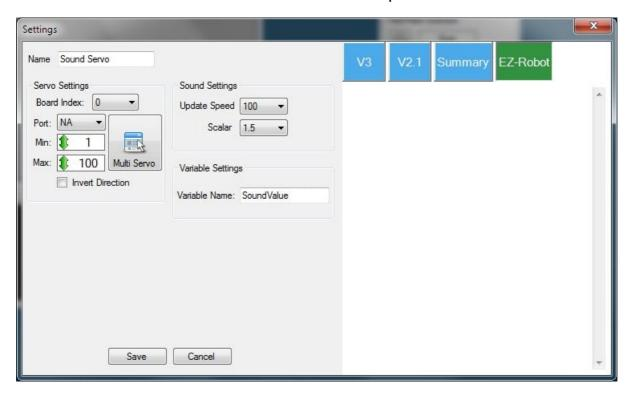
Notice how the port used is set to N/A. We don't want it to control any servo directly, what we want is the variable it gives.
