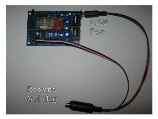
NOTE: Up to 22 vdc can be on the same power terminals if the Roomba is in a charging state. It is advisable to disconnect the EZ-B when charging the battery.
