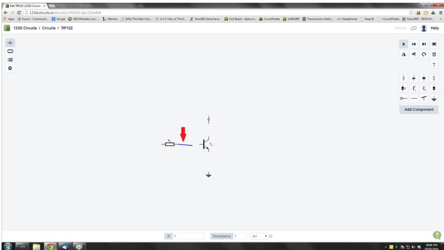
Add in the other components, nodes and circuit lines to complete the circuit. Then add in the labels for the nodes. To add the labels, or to change the values and part numbers of the components click on them, at the bottom of the screen the information will pop up, simply click in the box and adjust the text to suit.
