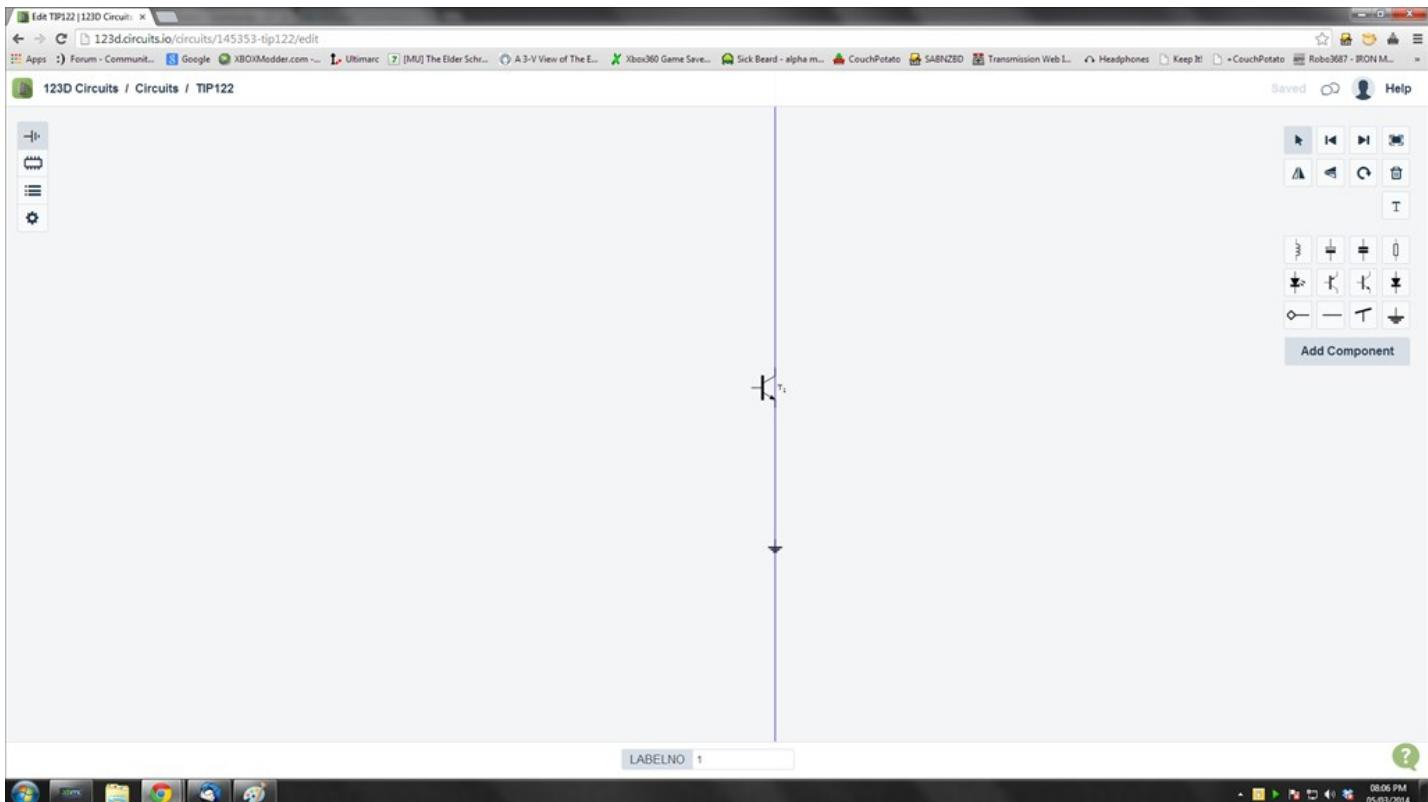
Next we add a node, which will be going to the item the transistor is switching, be it an LED, lamp, buzzer, motor or whatever, so select the node and place it down. The node will be at the wrong rotation so once it's placed down click on it to highlight it and select the rotate button from the pallet of tools.
