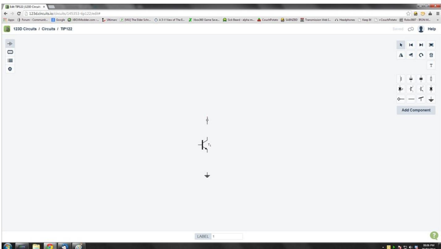
And now it's time to join it all up with circuit lines. To add these simply click on the end points of any of the components, a blue line will now be joined to the component and your pointer, then click where it needs to go to and the circuit line is added.
