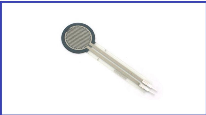
These sensors allow you to detect physical pressure, and can be used on things such as a robot claw to detect pressure and stop the claw servo from moving. (Pull up or Pull down resistors may be required. See the [Flex Sensor Tutorial](#) for details).
