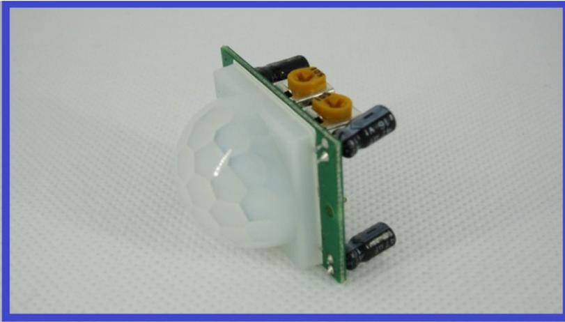
These little sensors measure infrared light, and can be used for motion detection. Some PIR sensor modules have the option to work on analog ports, or on digital ports as well.
