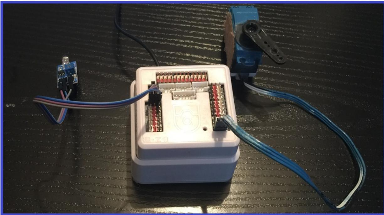
8.) Power on your EZ-B, and connect it to EZ-Builder. Now press "**Start**" on the script control, and the servo will now move when the sensor detects different brightness of light which change the analog readings. As an optional extra, you can add an ADC control like the "ADC Value" control seen in the video below, to see the sensor readings change as they happen. Check out the short video demo of this in action...
