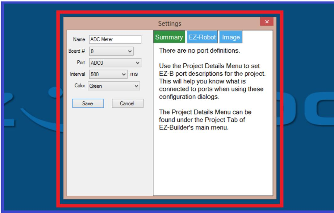
4.) Now connect the EZ-B to Ez-Builder, and make some noise... literally. The louder the sound is detected, the higher the visual display will go in the control window. You may need to adjust the potentiometer on the sound sensor to adjust the sensitivity.
