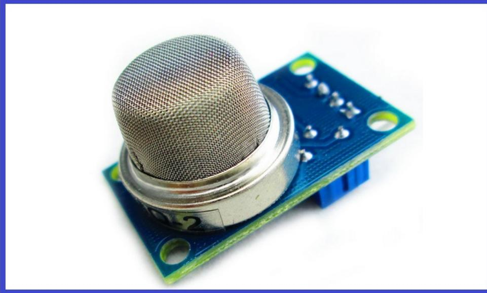
Can be used to detect smoke and other gasses, such as methane and butane gas.
