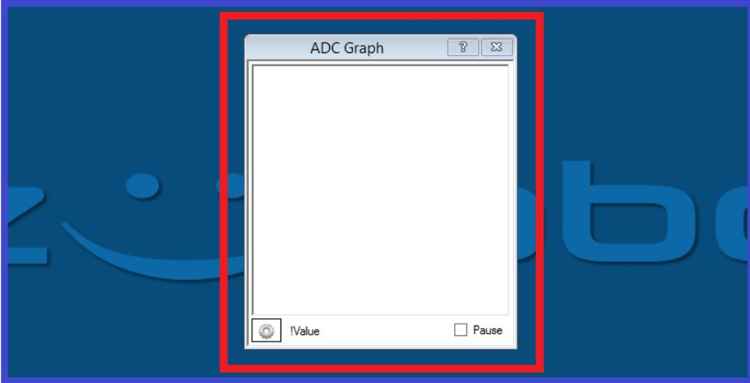
This control will show the ADC voltage in a historical graph. The input voltage can be between 0 volts and 3.3v. A demonstration of this control can be found in step 6.
