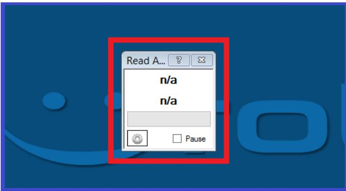
This ADC control will display a numeric value and voltage from the selected ADC port chosen that is chosen from the configuration menu. A demonstration of this control can be found in step 5.
