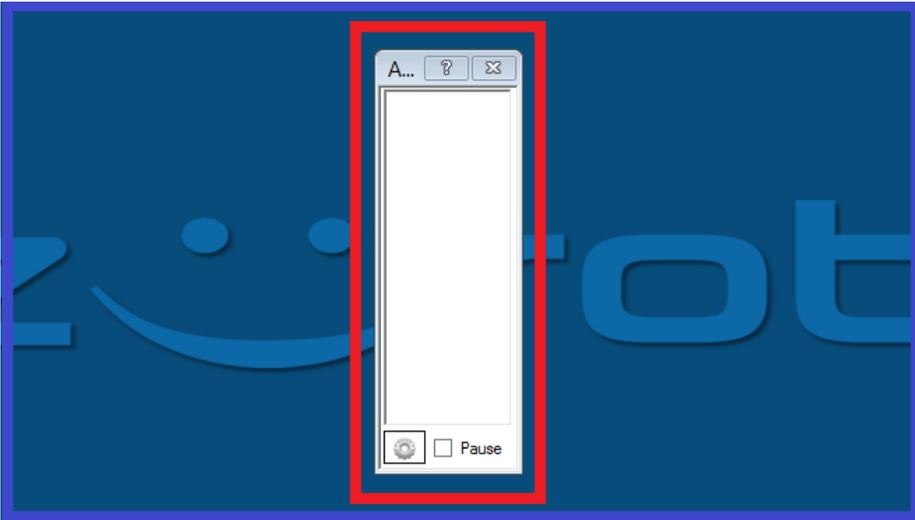
Displays the ADC (Analog Digital Converter) voltage in a VU (volume unit) meter. The voltage can be between 0 and 3.3v. A demonstration of this control can be found in step 7.
