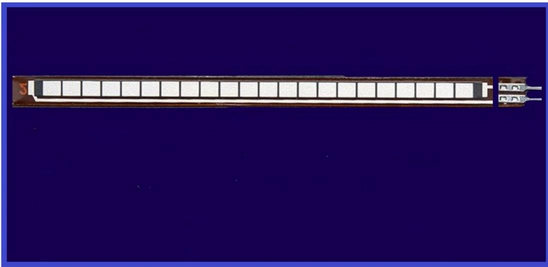
Much like the pressure sensors mentioned above, these can measure resistance and increase analog readings the further they are bent. What a look at the [Flex Sensor Tutorial](#) for more details and a video example.
