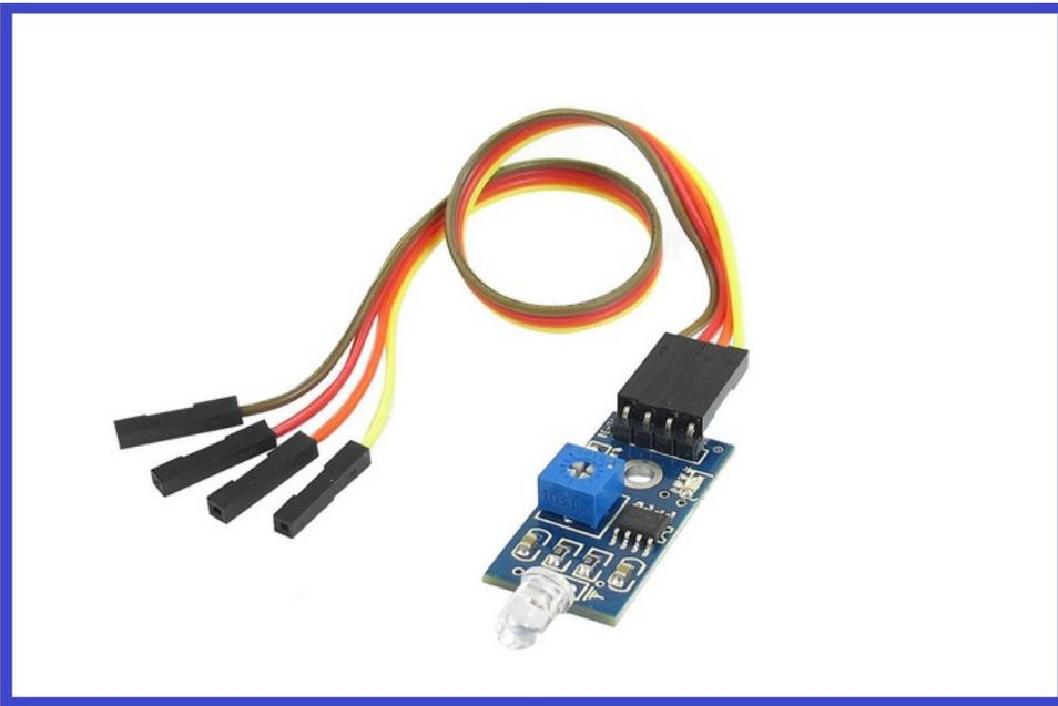
These detect "Light" and can be used for many applications. One example is to have one of these plugged in to your EZ-B, along with a low level spotlight. When the sensor levels change when in a dark room, this will trigger the spotlight to come on. (You can adjust the ADC values so the light from the spotlight doesn't cause the sensor to turn it off again).
