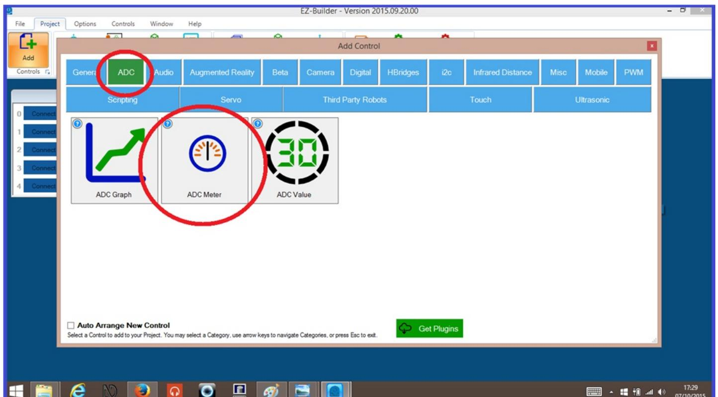
3.) On the "ADC Meter" control, click on the gear icon to open the configuration menu, and select the port the sensor is connected to, then click "**Save**".
