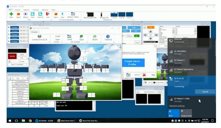
Select Connect to **EZ-B**. The robot should move into the initialization position.
