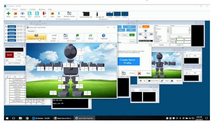
The servos of each arm and leg should be positioned in a straight line. Do not manually manipulate the servos when the robot is powered on.
