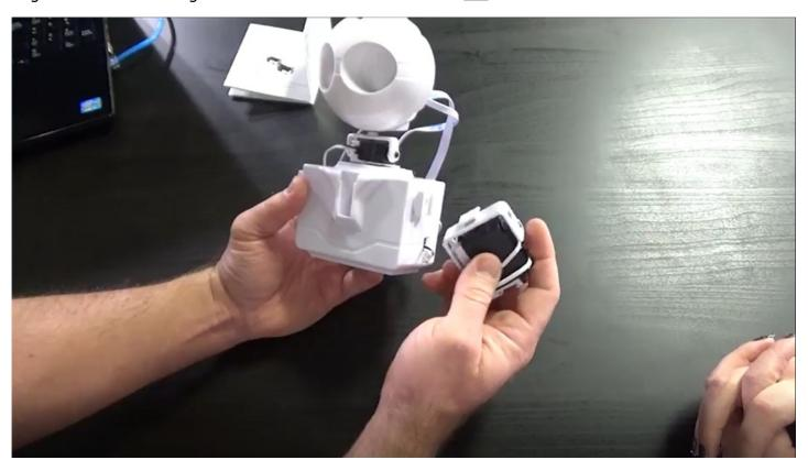
Clip'n'Play Left Forearm Servo to the Left Upper Arm Servo. Connect the cable to <u>D5</u>.
