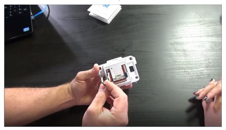
**EZ-Robot Clip'n'Play Technology** allows **EZ-Bits** to be connected using a simple pressure fit clip. Insert the male clip into the female side of the **EZ-Bit** and press together. To remove, reverse the process.
