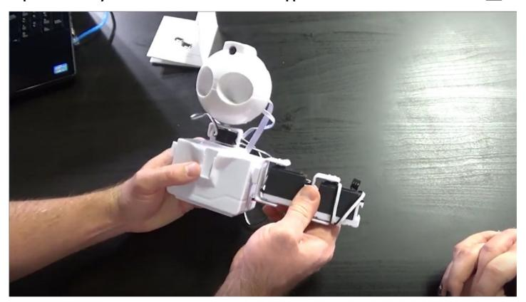
Clip'n'Play Left Gripper to the Left Forearm Servo. Connect the cable to  $\underline{\mathbf{D6}}$ .
