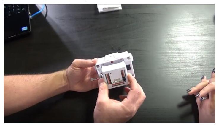
Connect the **Right Shoulder Servo** cable to  $\underline{\textbf{D2}}$  and **Left Shoulder Servo** cable to  $\underline{\textbf{D3}}$ . Match the black wire on the cable to the black side of the **EZ-B** port.
