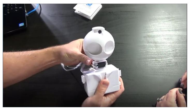
Connect the horizontal (left-to-right motion) servo to <u>DO</u>. Connect the vertical (up-and-down motion) servo to <u>D1</u>. Connect the **Camera** cable to the <u>camera port</u>. Connect the **RGB Eyes** cable to any of the <u>i2c ports</u>. Review the **Getting Started Guide** for a full diagram of the port configuration.
