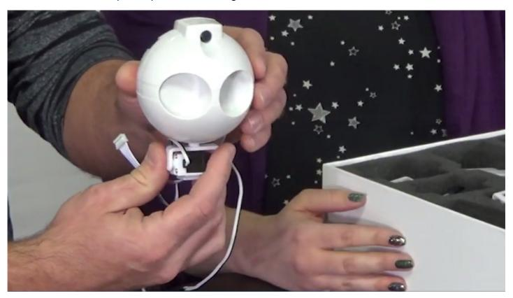
The **Humanoid Body** has two shoulder servos, which control rotational movement for the right and left shoulders. The body also houses the power switch and a contained **LiPo Battery**.
