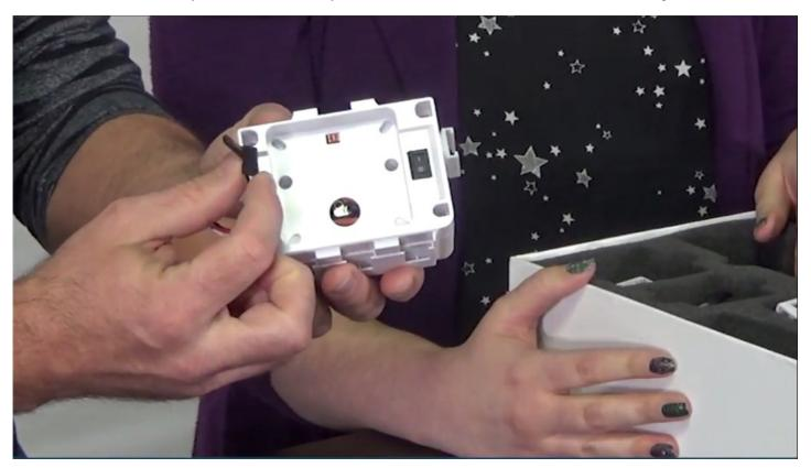
The **EZ-B v4 Robot Controller** houses an internal speaker and all of the connection ports. It acts as the processing brain for the robot. The controller connects to the computer using Wi-Fi.
