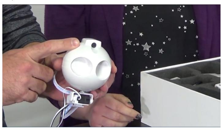
The **RGB Eyes** are a peripheral that can be programmed to show different colors and patterns. The **Head Assembly** uses servos to move horizontally and vertically. Servos are a type of motor that can be controlled for specific positions and angles.
