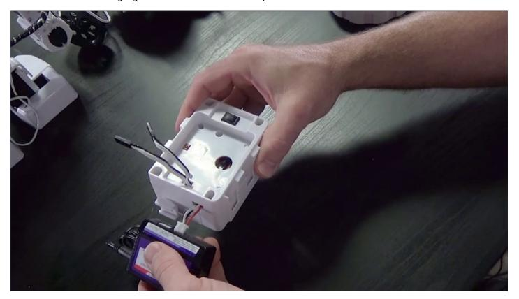
The  $\bf Revolution\ JD$  battery connection is under the left arm. Use your thumb and finger to securely connect the cable to the charger.
