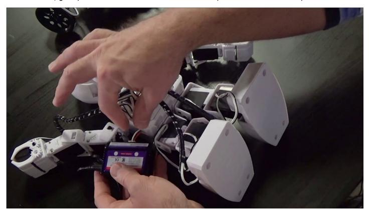
The  ${\bf Revolution}~{\bf AdventureBot}$  battery connection is located under the body.
