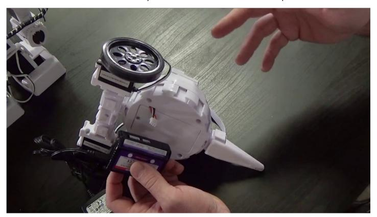
The Revolution Six battery connection is located under the body.
