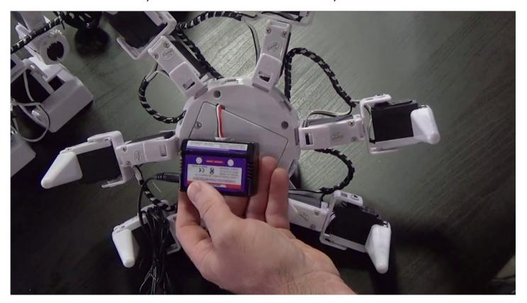
The **Revolution Roli** battery connection is located under the body. Lean **Roli** backwards for easiest access.
