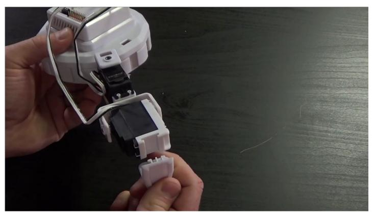
**Clip'n'Play** a **Lever Servo** into the "11 o'clock positionâ€.
