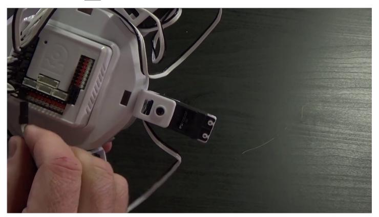
$\textbf{Clip\^{a}} \textbf{C}^{\text{\tiny{IM}}} \textbf{n\^{a}} \textbf{C}^{\text{\tiny{IM}}} \textbf{Play} \text{ the outside } \textbf{Lever Servo} \text{ with the white bracket on the left-hand side.}$
