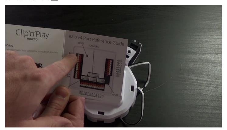
Match the black wire on the cable to the black side of the  $\bf EZ-B$  port. The cables use a male-to-female connection.
