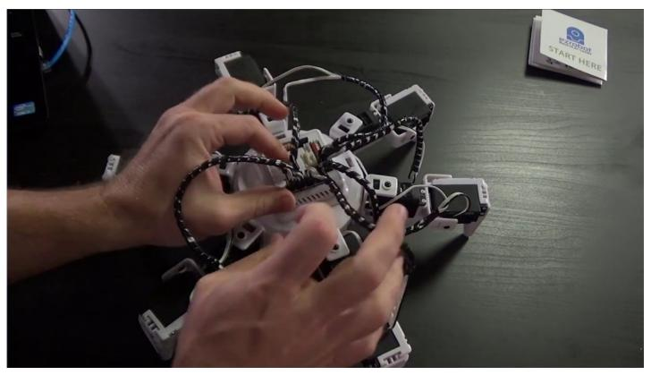
Check that connections are still secure and test for full motion.
