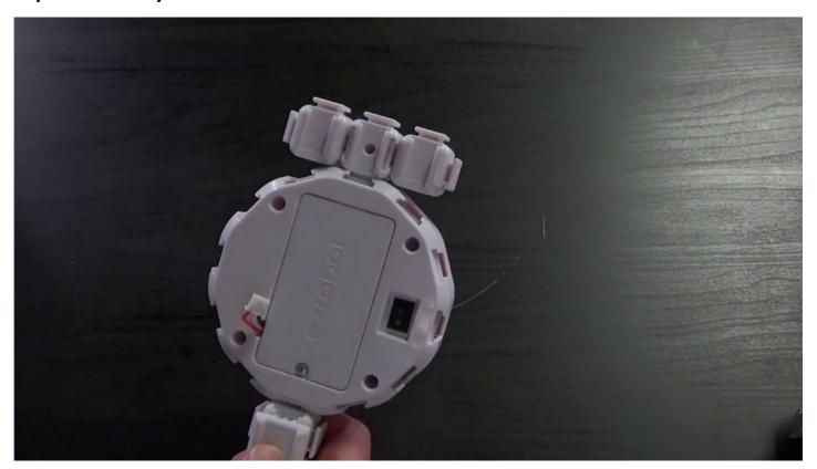
Clip'n'Play a Continuous Rotation Servo to the left Extension Cube with the white bracket toward the inside.
