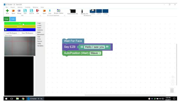
Once the robot detects a face, it will speak and complete the wave action.
