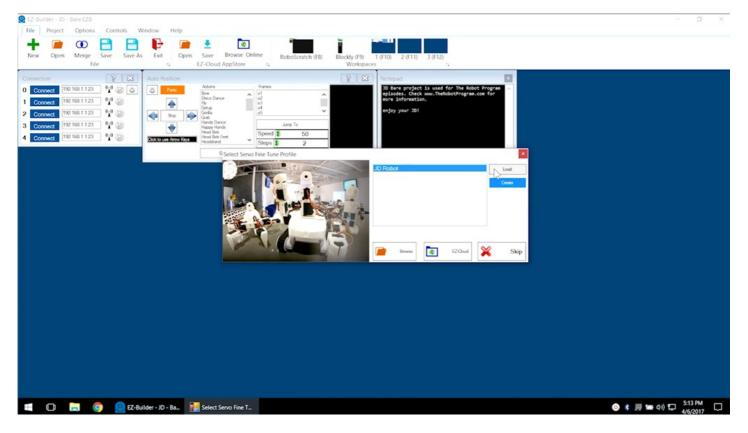
Power on the fully charged robot. Use Wi-Fi to connect to the EZ-B and click on the blue **Connect** button.
