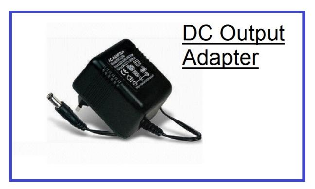
These have various choices of voltage and current output, and have transformers built in to them which are mainly (but not always) unregulated, meaning that the output is not guaranteed to be a specific value, but it will be at least what is says on its specifications. For example, with a 9v adapter drawing 300mA, the voltage is guaranteed to be higher than 9V.
