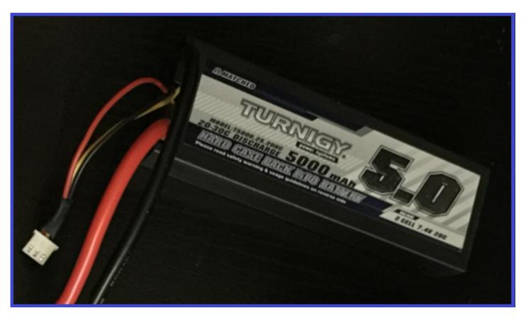
lithium-ion polymer batteries tend to be flat cells but can be made in almost any shape, and are usually found as multiple packs of 3.7 volt single cells. As with other batteries, they come in different flavours of voltage...
