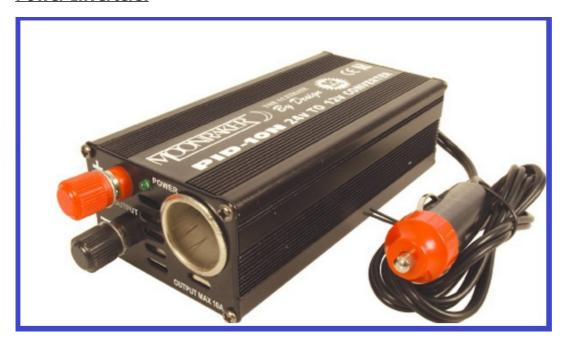
A power inverter is designed to convert DC to AC. For example, the input power to the inverter would be a DC source from a battery. This is then converted to AC, so an AC powered device like a TV that is usually powered from the mains supply, can operate. The efficiency of many inverters is around the 80% mark and sometimes have built in low battery voltage protection.
