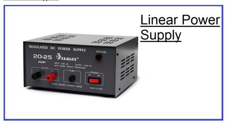
Compared to the different type of power supply adapters mentioned so far, these are more recommended. A linear power supply uses simpler electronic designs than switching supplies, but need much more cooling that makes them less efficient. This is because they use bulky transformers to convert the power. Linear power supplies operate with only around 50% efficiency due to energy lost of heat which is lost using large heat sinks.
