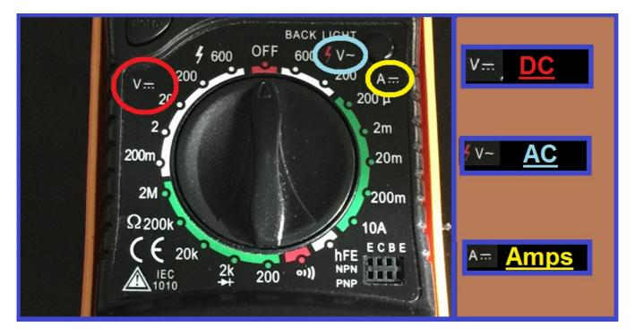
Some multi-meters are auto ranging, but this one is done manually, so it has different voltage ranges for DC on the left of the meter, and AC on the right...
