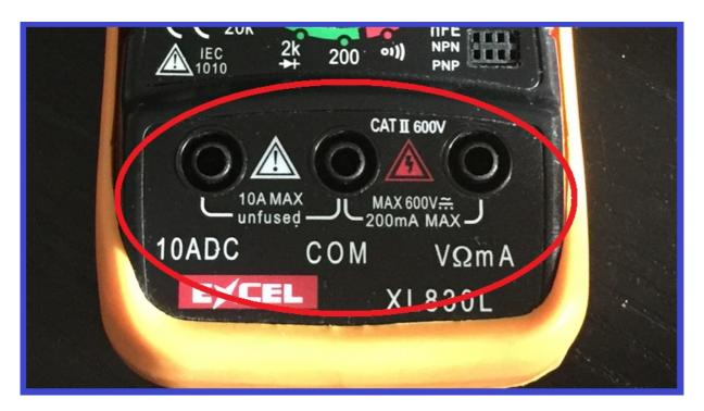
**10 ADC** Can measure up to 10 amps before the fuse between the "10ADC" and "COM" terminals blows if the 10 amp limit is exceeded.
