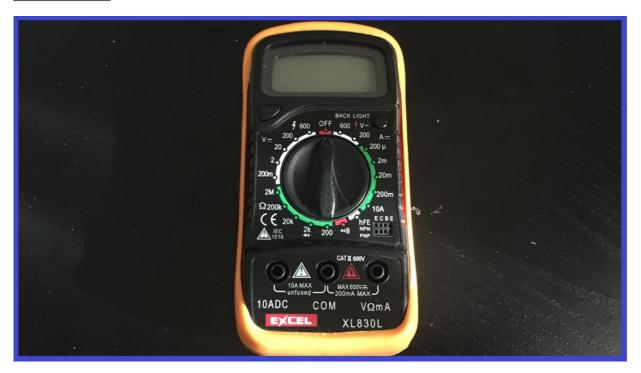
A device that has the options to measure both voltage, and amperage. Basically, the two meters mentioned above, in one unit. They can also measure resistance.
