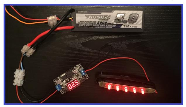
In the image, the setting is an output for 2.5v which is fine for powering 3v LED's. If you think about it, LED's powered by two alkaline batteries in series will not always get the full 3 volts on offer, as the alkaline's slowly deplete as they are used.
