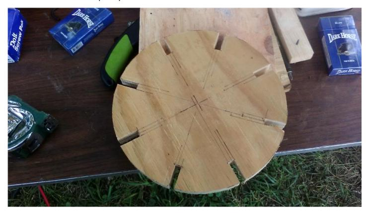
Take your time cutting the wheel out, because everything must be as square as possible. If you need to do any sanding, now is the time to do it, but don't paint or seal it yet. This is also the time to drill any holes, cut slots, etc. to lighten up the wheel. Just don't cut into the hub area, and leave at least an 1 1/4 inch rim around the outside undisturbed, because of the screws used to mount the tire to the wheel.
