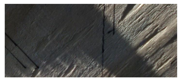
Here is how I laid out the slots for bracing. They are 3/8 inch wide, by 1/4 of the radius deep, in this case 1.25 inches. Measure and cut them as accurately as possible, because they will be glued in, and they are a major part of what keeps your wheel true and square.
