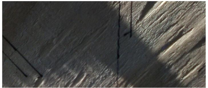
Here is how I laid out the slots for bracing. They are 3/8 inch wide, by 1/4 of the radius deep, in this case 1.25 inches. Measure and cut them as accurately as possible, because they will be glued in, and they are a major part of what keeps your wheel true and square.
